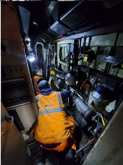
Right: Finally, Ben and Steve refitting parts to the brake frame. Much of this had been robbed to keep other power cars going. But we've managed to find most of the parts to fit back on and make the power car moveable on the mainline again hopefully in spring, albeit not under its own power.....yet!
