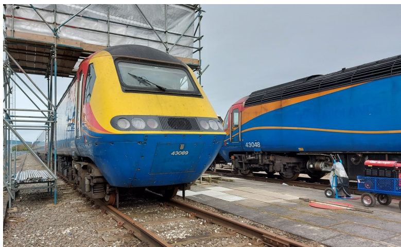
Left: 43048 & 089 standing side by side at Rectory whilst Ben and James attend to their needs on February 14th prior to their outing the following week. Note the generator and battery charger being used to help them into life. © James Trebinski
